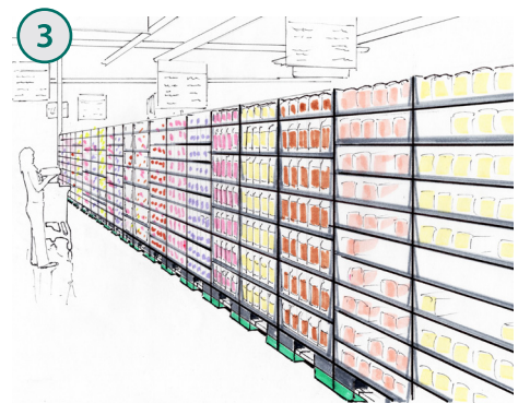
3 Place loads on retail floor for easy replenishment. Customers shop directly from trays.
